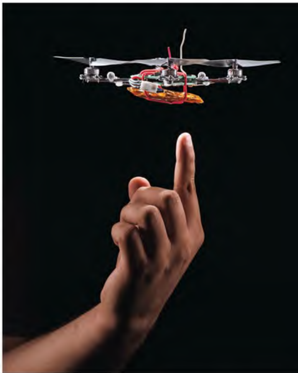
This “micro air vehicle” with four rotors, made by KMeI Robotics in Pennsylvania, can fly in swarms with its mates. The drones navigate autonomously, without a pilot.
